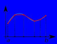
The area of each strip (trapezium is found separately. Hence the area under the curve y = f(x), between the lines  $x = x_0, x = x_n$  is approximately equal to the sum of the area of the *n* trapeziums.
